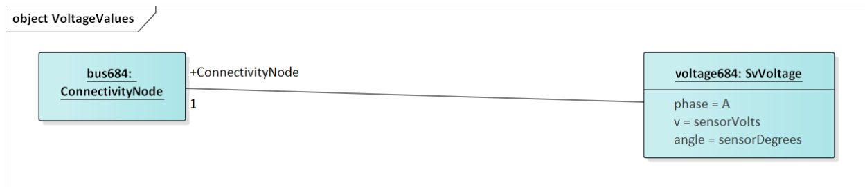
Figure 39: In this profile, a solved voltage value attaches to ConnectivityNode in GridAPPS-D. Positive sequence or phase A is implied, unless the phase attribute is specified.
